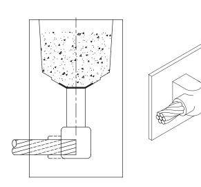
**CS-31**Place end of cable to center of tap hole. Secure to surface using B-106-41 chain clamp or a C-Clamp.
