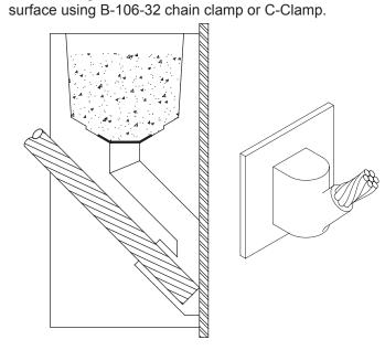
Butt cable against steel surface as shown and secure to
